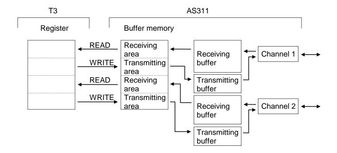
Here, a message (one set of transmission characters) means a string of ASCII characters which is ended by specified trailing code. The default setting of the trailing code is CR (carriage return code = H0D).
